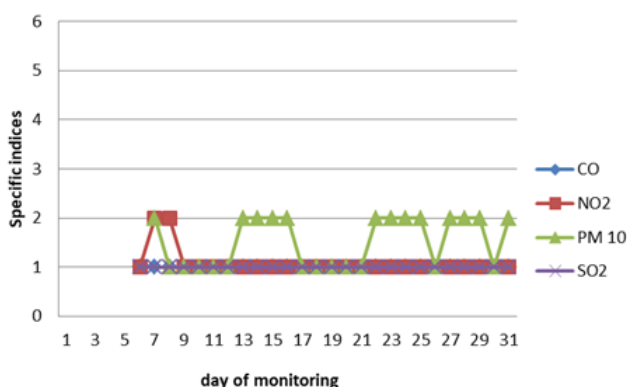
Fig. 5. Specific indices corresponding to the concentration level of monitored pollutants
